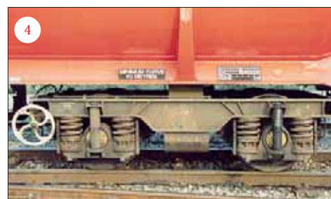
Photos 1-6 show PR85313, captured on film at the Westerleigh distribution terminal. 2: discharge pipework detail. 3: buffer over-ride protection plate (fitted to most vehicles). 4: side view of Schlieren pattern bogie fitted with additional dampeners. 5 & 6: air brake detail. 7: end view of PR85313 at Hereford, showing ladder access detail. 8 & 9: tank roof vents and filler cap detail. Photographs and drawing by the author.
