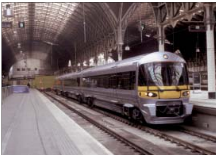
Above: platform 7 at Paddington on 24 April 1998, with Heathrow Express unit No. 332 010 awaiting departure. The unobtrusive way in which the 25kV overhead live equipment was installed for these trains is worthy of note.
