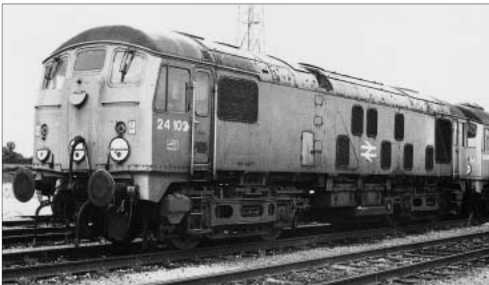
Above: 24 102 (Darlington, 1960) at Carlisle Kingmoor on 1 August 1977, 18 months after withdrawal. One of a batch converted for use on Tyne Dock-Consett ore trains, it has minor differences from Cambrian 24s but the photo shows clearly the cab and dome roof profile. Photograph: Ian Futers.
