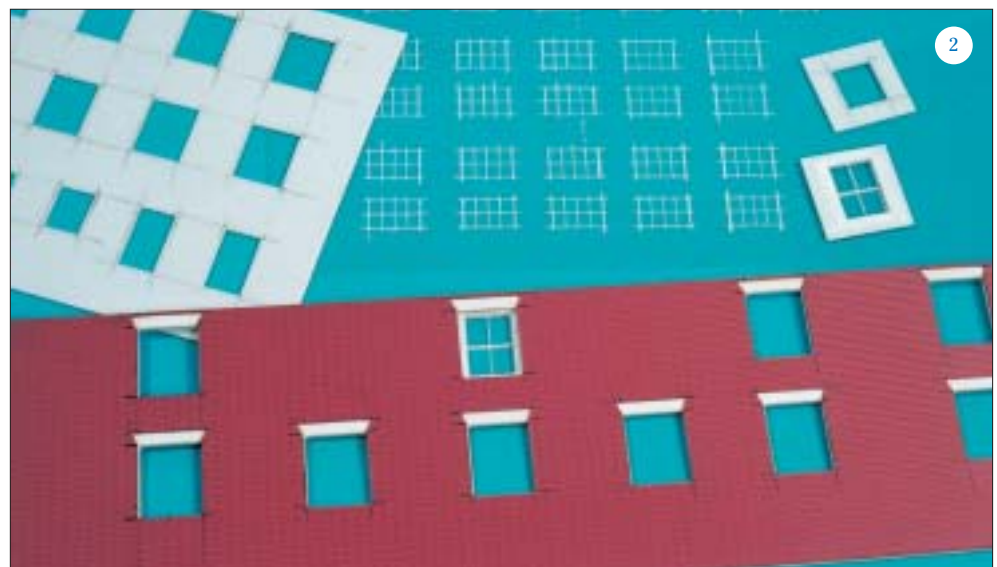
Photo 2: the component parts of windows are shown here. Frames are cut from plastic sheet with glazing bars painted on to clear plastic sheet. Note that the frames are not fitted until the wall colouring is complete; the single frame shown in the wall side has only been positioned temporarily for this photograph.
