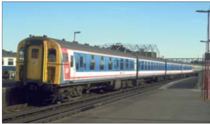
Above: a Southern innovation of the highest order – electric traction on the country's first electrified main line, the former LBSCR. NSE-liveried 4-CIG No.1921 trails a Victoria-bound service on 22 September 1987.
