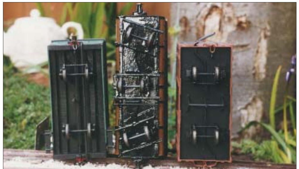
Below: underside views of WHR No.2, FR No.2 (described November 03 issue) and FR Cleminson open. On the model Cleminson the chassis differs slightly as the end 'wheelset' guides are fixed on to the wheelset, not the solebars. This makes the model chassis more flexible again. The photo also shows the brake and pipe gear on the two brake vans.
